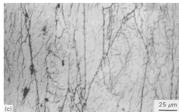
Figure 1 (a) Typical macrostructure of an EB weldment; (b) microstructure of this weldment, and (c) a higher magnification of weld metal after oxalic acid etch test.
